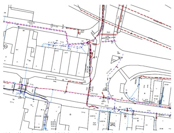
High and low voltage National Grid electricity services run in the pavement and carriageway around Eastern Gateway. The area suggested as the cycled hub café does not appear to have many services running in it, although some HV and LV services appear to run in the pavement on the North side of lower fore street. Some of the proposed planting to Fore Street may clash with some LV services however the electrical buried services in these locations to do not look to be too extensive.
